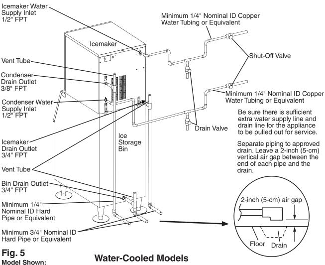
Connection to an Open Drain System
